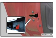
• To enter the vehicle, unlock the driver door by mechanical key. After entering the vehicle, operate the inner handle twice to unlock other doors.
