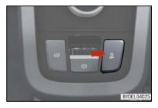
When ESP system is turned off, if ESP OFF switch is pressed again or the driving speed exceeds the threshold (80Km/h), some functions of the turned-off ESP system will be turned on again. In order to avoid the sudden opening of ESP system functions, ESP system function can only be reactivated if ESP system is not in the dynamic intervention status of the car.
