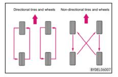
While purchasing replacement tire, you may find out Some tires are directional and can be used for tire rotation only along one direction. For the use of directional tires, swap the front tires with rear tires only during the tire rotation, as shown in above diagram.
