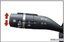
When the turn signal is turned on, the turn signal will be flash even if letting it go. After the turning operation is completed, the turn signal and the turn indicator on the dashboard will be turned off. Depending on the driver's operating habits, it's necessary to rotate for one turn to return under individual extreme case.
