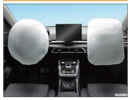
The vehicle is installed with driver airbag and front passenger airbag. When the airbag system ECU detects a medium or severe frontal impact during traveling and the airbag triggering conditions are met, the airbag will deploy to supplementally protect the head and chest of driver/front passenger, in order to mitigate the injury extent of the driver/front passenger.
