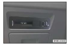
The illumination height of the headlamp is the maximum when the headlamp adjustment switch is at 0 position and is the minimum when the headlamp adjustment switch is at 5 position. Depending on the driver's need, adjust the switch to any of 0~5 positions to change the illumination height of the headlamp.
