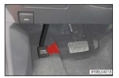
Release of parking brake: Depress the brake pedal by right foot to prevent vehicle gliding and depress the parking brake pedal forcibly by left foot and then release to restore the parking brake pedal to initial position. The instrument icon of parking brake indicator lamp disappears and the parking brake is released.
