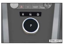
Gear P is the parking gear. Press the gearshift knob button to realize parking. The indicator lamp on the button turns on. Shift to this gear before starting or stopping the vehicle. Depress the brake pedal to start the vehicle and then shift from gear P to other gear (If fitted).
