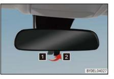
Anti-glare mode - Place the lever in Position 2, in the position, the glare from the headlights of coming cars can be reduced effectively at night. It should be noted that while the glare is reduced, the sharpness of the rear view may be degraded.
