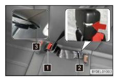
After unlocking the small tab, assemble the small tab to the cover plate 3.
