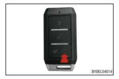
After successful start, press and hold "Start/Stop" button on the electronic remote key for 2s, the car will be shutdown, the power switch will be turned to "OFF" position, and the turn signal will flash twice.
