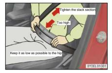
Insert the latch into the buckle until a click is heard, and pull the latch in the opposite direction to confirm that the seatbelt is locked successfully. Note that the seatbelt cannot be twisted.
