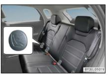
The outer rear seats are provided with anchorages (for top tether).
