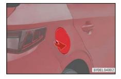
Open the charging coupler protective flap of vehicle and ensure that there is no obstacle on the ends of charger or charging coupler.
